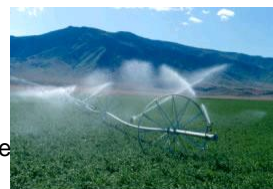
Wheel line Sprinkler System
