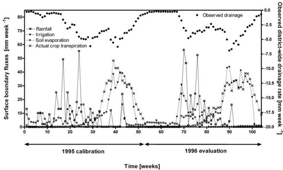
**Figure 3.** Weekly calculated soil surface boundary conditions for 1995 and 1996 (time 0 corresponds to 1 October 1994). Also included is the spatially averaged weekly measured drainage data of the BWD.
