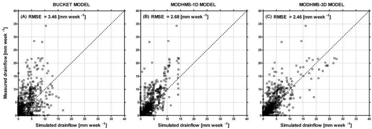
**Figure 13.** Case II-validation: Scatterplot of simulated versus observed drain flow values for all drainage units, when assigning different parameter sets to each unit using the (a) BUCKET, (b) MODHMS-1D, and (c) MODHMS-3D models.
