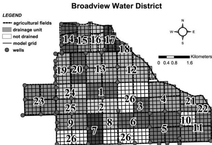
**Figure 2.** Schematic overview of the BWD. The numbers refer to individual drainage units, which may consist of a single field, two adjacent fields, or all four agricultural fields in a 1.6 km by 1.6 km (1 mile<sup>2</sup>) land section.
