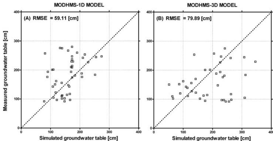
**Figure 14.** Case II cross validation: Scatterplot of drainage unit average simulated groundwater table depths versus observed values using the (a) MODHMS-1D and (b) MODHMS-3D models.
