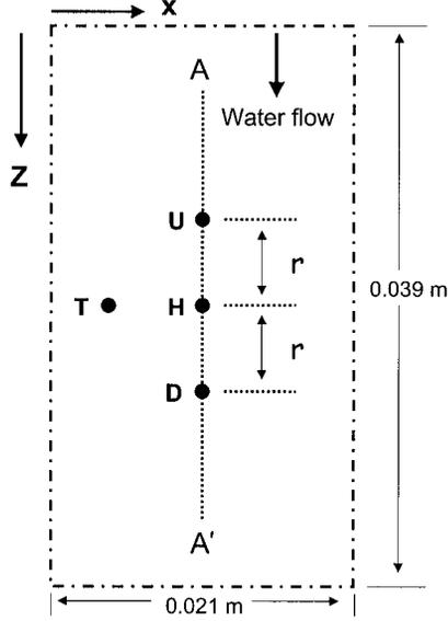
**Figure 2.** Simulated soil domain showing front view of heater needle (H), downstream (D), upstream (U), and transverse (T) sensors. Water flow direction is downstream.
