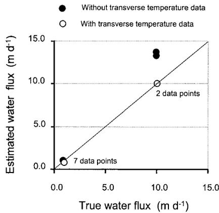
**Figure 8.** Comparison of estimated with “true” flux density values without (solid circles) and with (open circles) inclusion of the transverse (T) temperature data in the objective function (experiment II).
