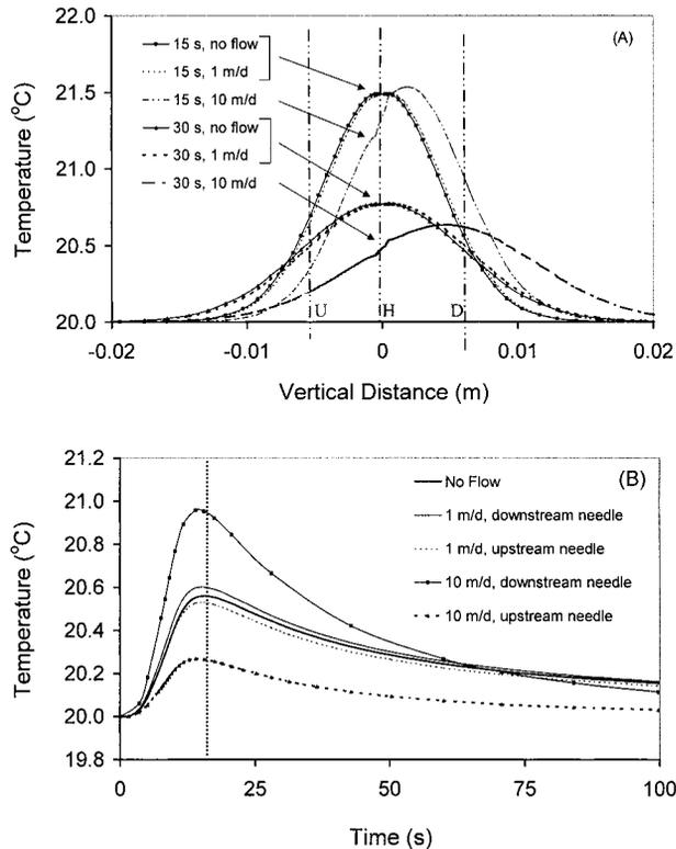
**Figure 4.** (a) Simulated spatial temperature distributions, 15 and 30 s after heating, for  $q_w$  values of 0, 1, and 10  $\text{m d}^{-1}$  (b) Simulated temporal distributions at the upstream (U) and downstream (D) temperature sensors for  $q_w$  values of 0, 1, and 10  $\text{m d}^{-1}$  (no thermal dispersion).
