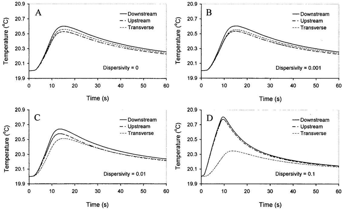
**Figure 5.** Temperature as a function of time for upstream, downstream, and transverse thermocouple locations for dispersivity values of (a) 0.0, (b) 0.001, (c) 0.01, and (d) 0.1 m ( $q_w = 1.0 \text{ m d}^{-1}$ ).
