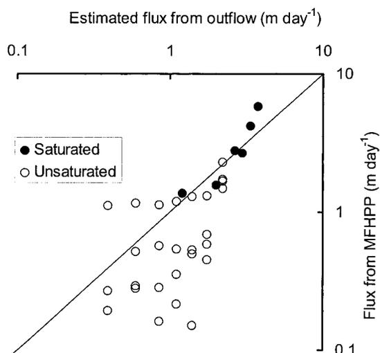
Fig. 11. Comparison of measured (multi-functional heat pulse probe [MFHPP]) with simulated water flux (SFOPT) values in the center of the flow cell for various multistep outflow experiments.
