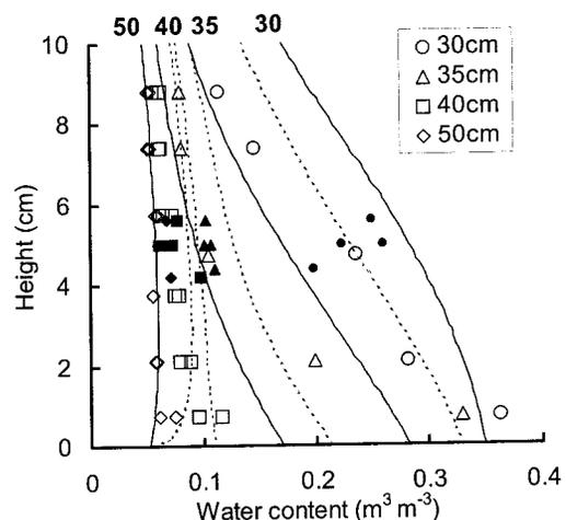
Fig. 10. Variation of  $\theta$  with height in flow cell as determined from gravimetric (open symbols), SFOPT simulations (solid and dashed lines), and MFHPP data (solid circles) for the indicated suction values.
