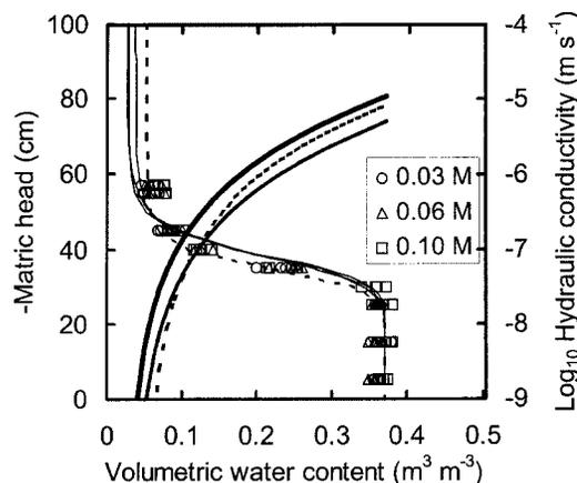
**Fig. 4. Optimized soil hydraulic functions. The symbols correspond with measured soil water retention data at the hydraulic equilibrium stages of Fig. 3, using the multi-functional heat pulse probe (MFHPP) and tensiometer data.**
