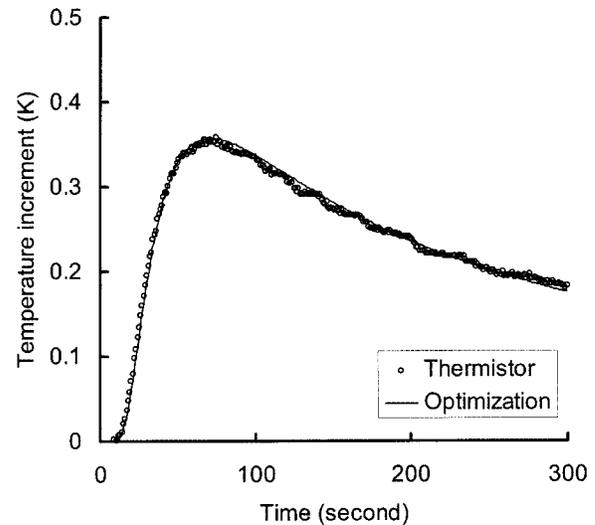
Fig. 6. Measured and optimized temperature response for the estimation of  $r_{\text{eff}}$  in agar solution.
