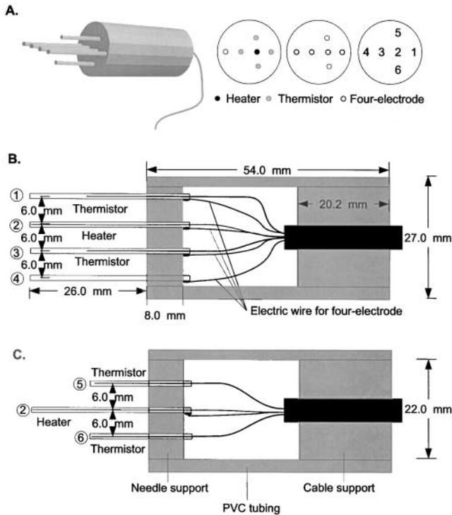
Fig. 1. Design of multi-functional heat pulse probe (MFHPP).
