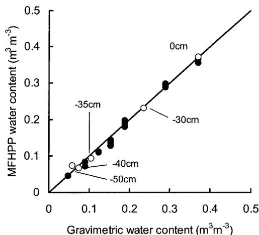
Fig. 9. Comparison of  $\theta$  measurements with multi-functional heat pulse probe (MFHPP) and gravimetric method. Solid circles indicate glass jar experiments; open circles denote the multistep outflow experiments.
