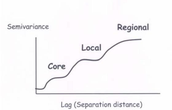
**Figure 2.** Hypothetical variogram for scale-dependent hydraulic conductivity. Adapted from Gelhar, [1986].
