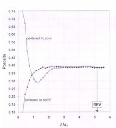
**Figure 4b.** Estimated porosity for a cubic domain with increasing size within the glass-bead pack [after Clausnitzer and Hopmans, 1999].
