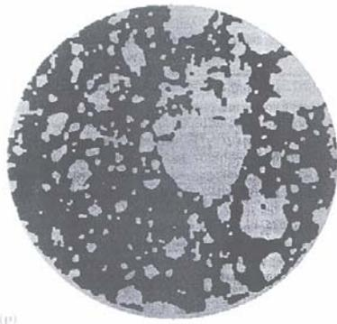
**Figure 5.** Illustration of two soil density classes in one specific cross-section of a 16-cm soil core [after Kasteel *et al.*, 2000].
