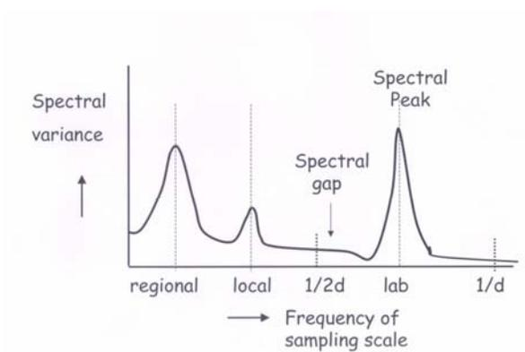
**Figure 3.** Schematic presentation of power spectrum, showing various process scales ( $d$  = sampling spacing).
