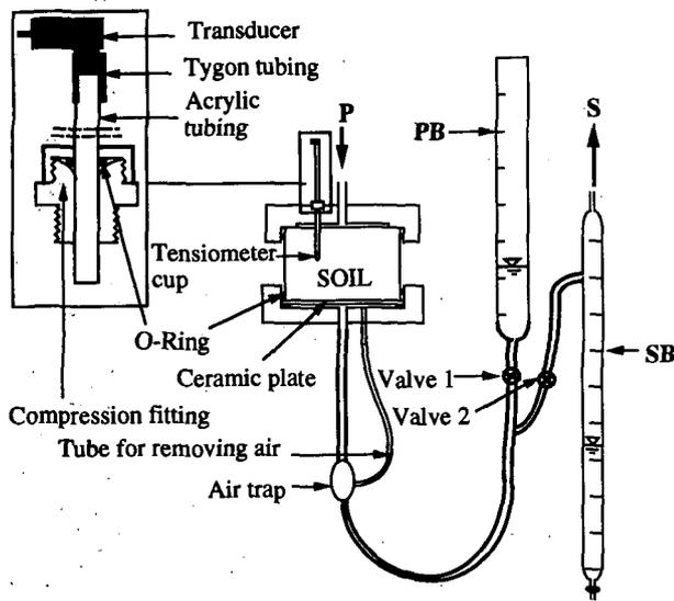
Fig. 1. Modified pressure cell (P, pressure inlet port; S, suction inlet port; PB, burette for pressure experiment; SB, burette for suction experiment).
