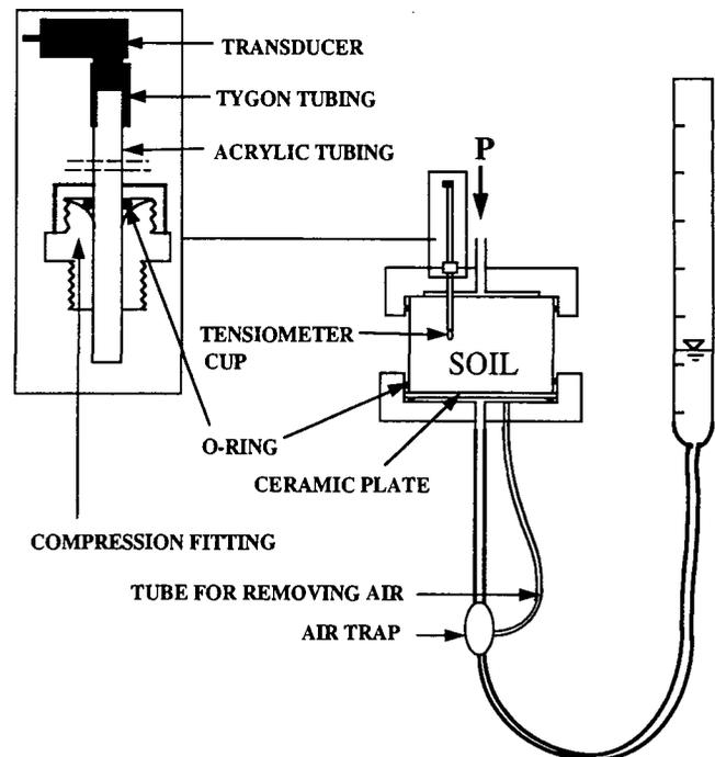
Fig. 1. A Schematic representation of the modified Tempe pressure cell for the multistep experiments.
