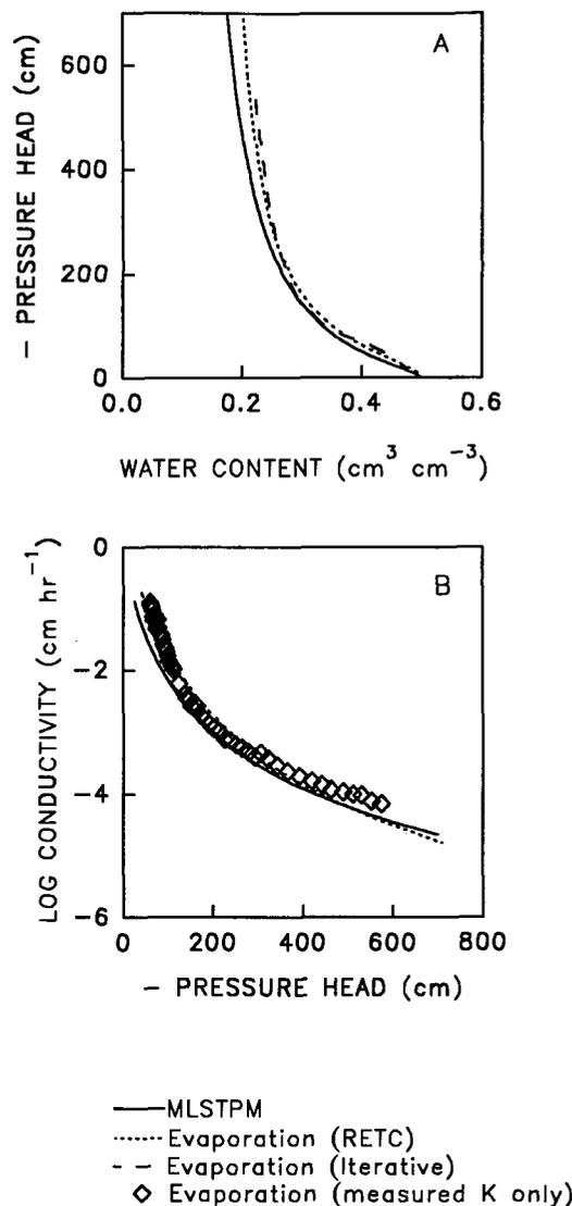
Fig. 5. (A) Soil water retention curves and (B) hydraulic conductivity curves for Panoche loam from MLSTPM and evaporation methods.
