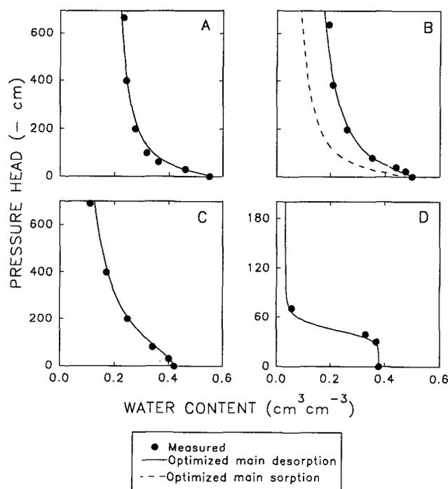
Fig. 2. Soil water retention curves for (A) Yolo silt loam, (B) Panoche loam, (C) Hanford sandy loam, and (D) Oso Flaco fine sand.
