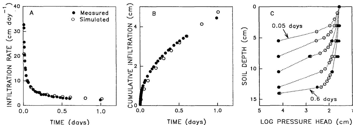
Fig. 6. Experimental and simulated (A) infiltration rate, (B) cumulative infiltration, and (C) pressure head profile for Panoche loam.
