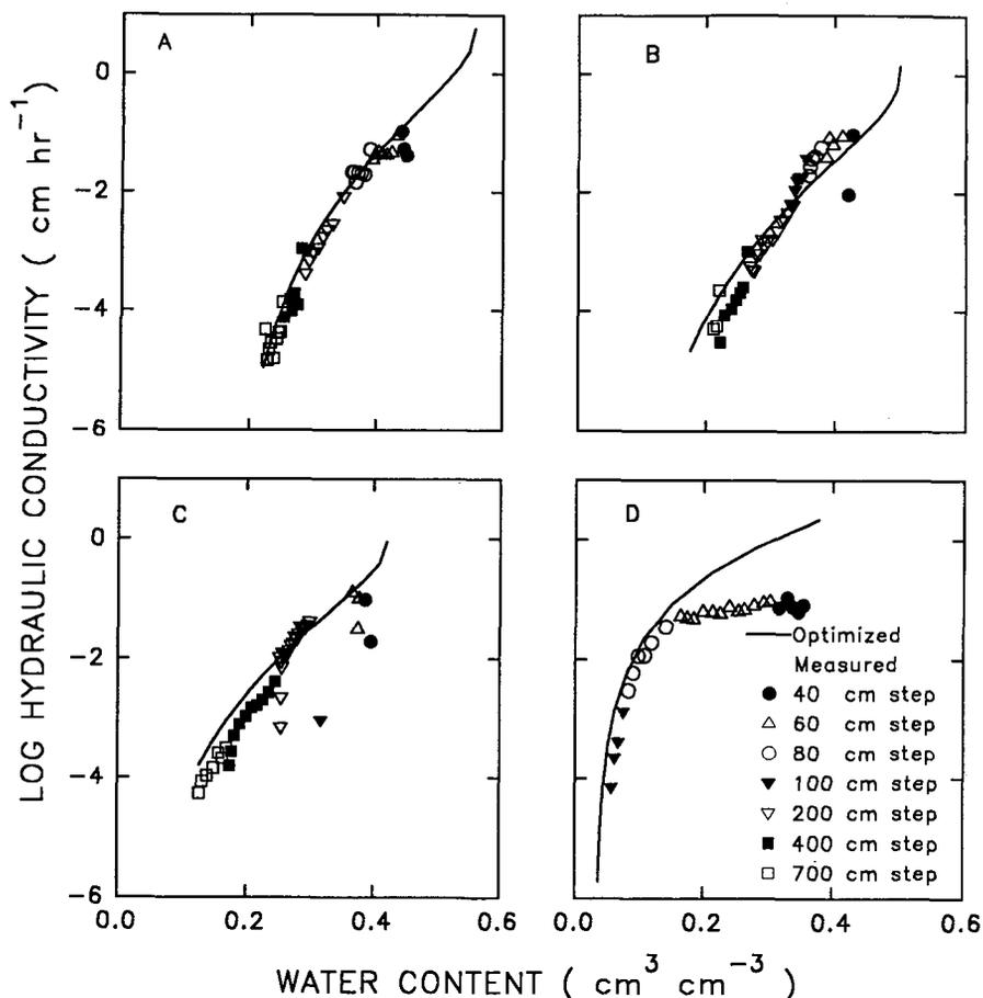
Fig. 4. Hydraulic conductivity curves for (A) Yolo silt loam, (B) Panoche loam, (C) Hanford sandy loam, and (D) Oso Flaco fine sand.
