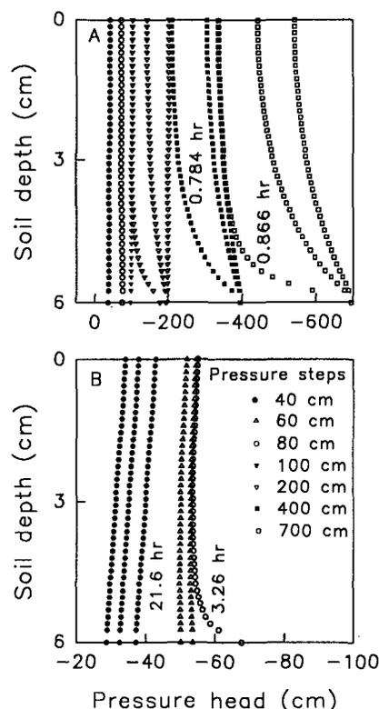
Fig. 3. Simulated soil water pressure head profiles at selected times for (A) Panoche loam and (B) Oso Flaco fine sand.
