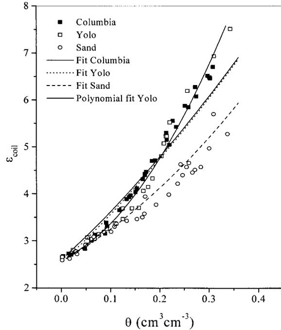
Fig. 6. Calibration data for the coiled TDR probe using Eq. [3] for all three soil types (from average values of bulk density and porosity in Table 1), using parameters  $n$ ,  $w$ ,  $\epsilon_{probe}$  fitted to Eq. [1] and soil specific  $\alpha$  values fitted to Eq. [2]. Fitted polynomial ( $\theta = -0.2977 + 0.1443\epsilon_{coil} - 0.00824\epsilon_{coil}^2$ ;  $r^2 = 0.963$ ) is used for field measurements.
