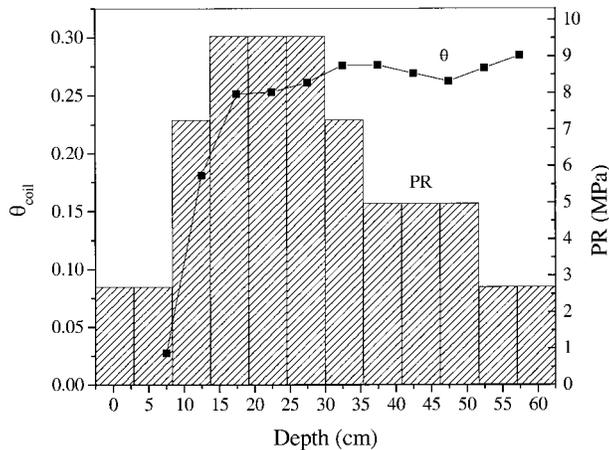
Fig. 7. Combined field measurement results of penetration resistance (PR) and water content ( $\theta$ ) obtained with the combined coiled time domain reflectometry (TDR)-cone penetrometer probe for the Yolo soil.
